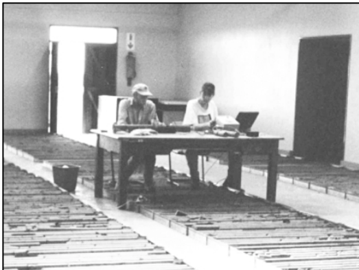
Figure 1 (left). Lew Ashwal and Sue Webb measuring magnetic susceptibility on 2950 meters of Bellevue core (image courtesy of the South African Journal of Geology)
